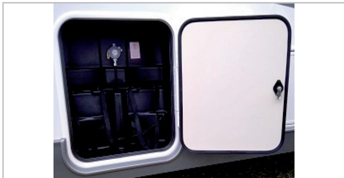
Fig.6.26 - Gas cylinder compartment
